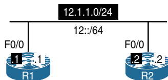
Figure 12-9 Configuring Match IP DSCP/Precedence vs. Match DSCP
