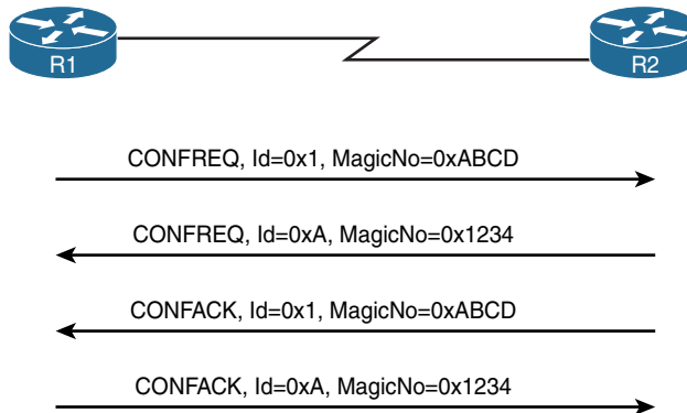
Figure 4-2 Basic LCP Message Exchange Between PPP Peers
